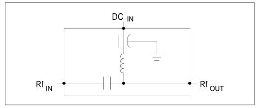
**Schematic Diagram (K and V Connector Models)**
