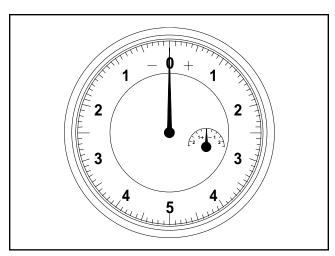
Figure 2. Pin Depth Gauge
